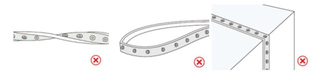
When installing the Flexi-Graze DO NOT twist, fold or bend sharply, all of these actions will damage the product.
