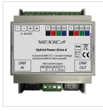
Hybrid Drive 6 is a versatile 'all-in-one' constant voltage LED driver that provides 6 channels of PWM output, from a supplied voltage range of 12-48VDC, or a DMX to SPI data conversion output to control dynamic pixel technology.
